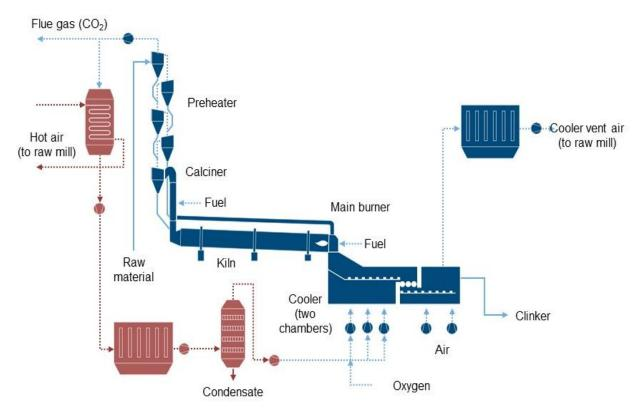
Schematic diagram of a 1st generation oxyfuel cement plant
