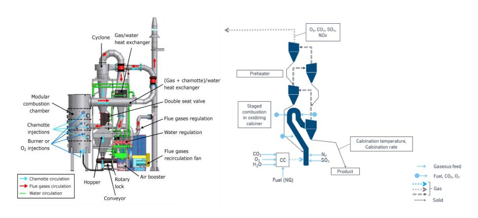
Schemes of pilot scale oxyfuel calciner facility from Air Liquide & TKIS
