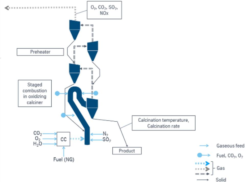
Schemes of pilot scale oxyfuel calciner facility from Air Liquide & TKIS
