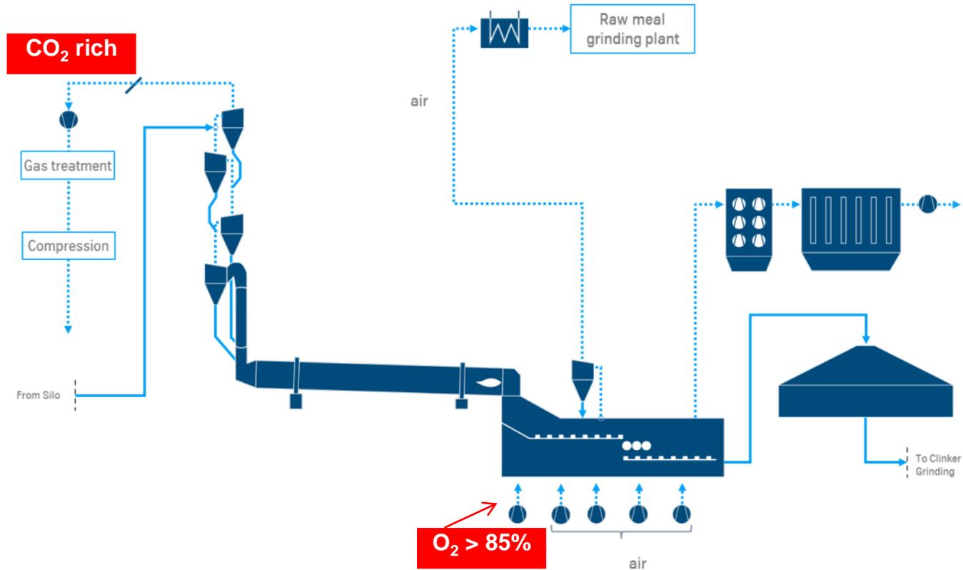
Schematic diagram of a 2<sup>nd</sup> generation oxyfuel cement plant without flue gas recirculation circuit
