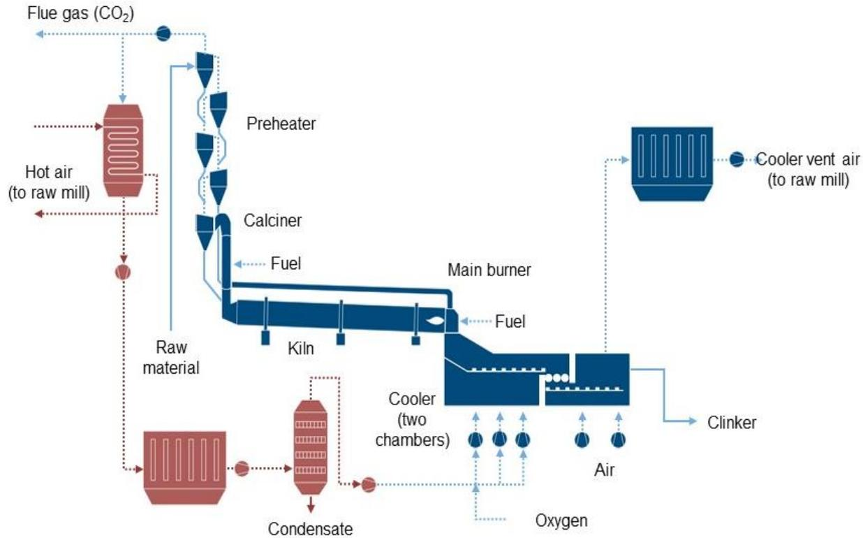
Schematic diagram of a 1<sup>st</sup> generation oxyfuel cement plant
