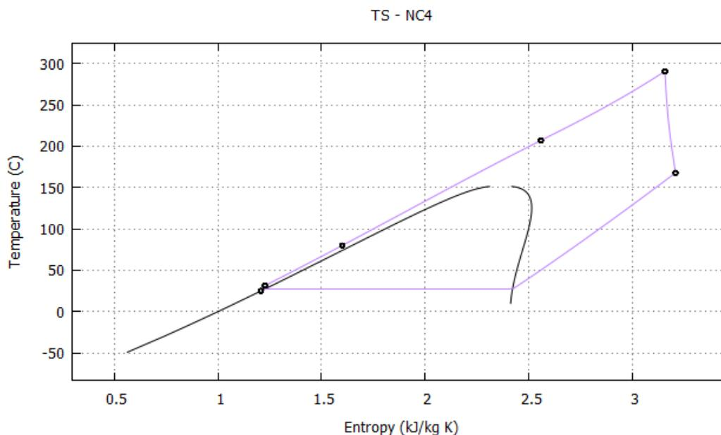
**Figure 25. T-s diagram of ORC using butane.**
