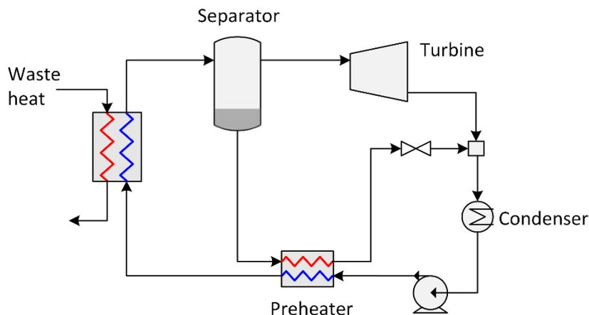
**Figure 12. Schematic diagram of a basic Kalina cycle.**
