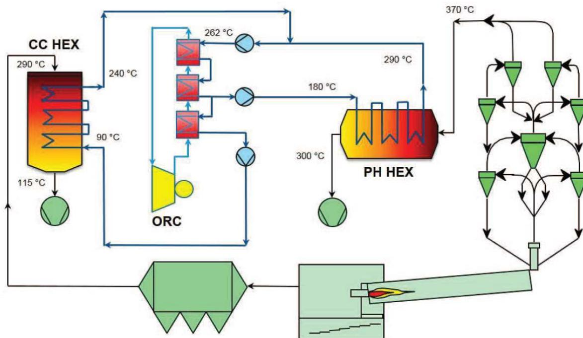
Figure 18. ORC waste heat recover system [55].
