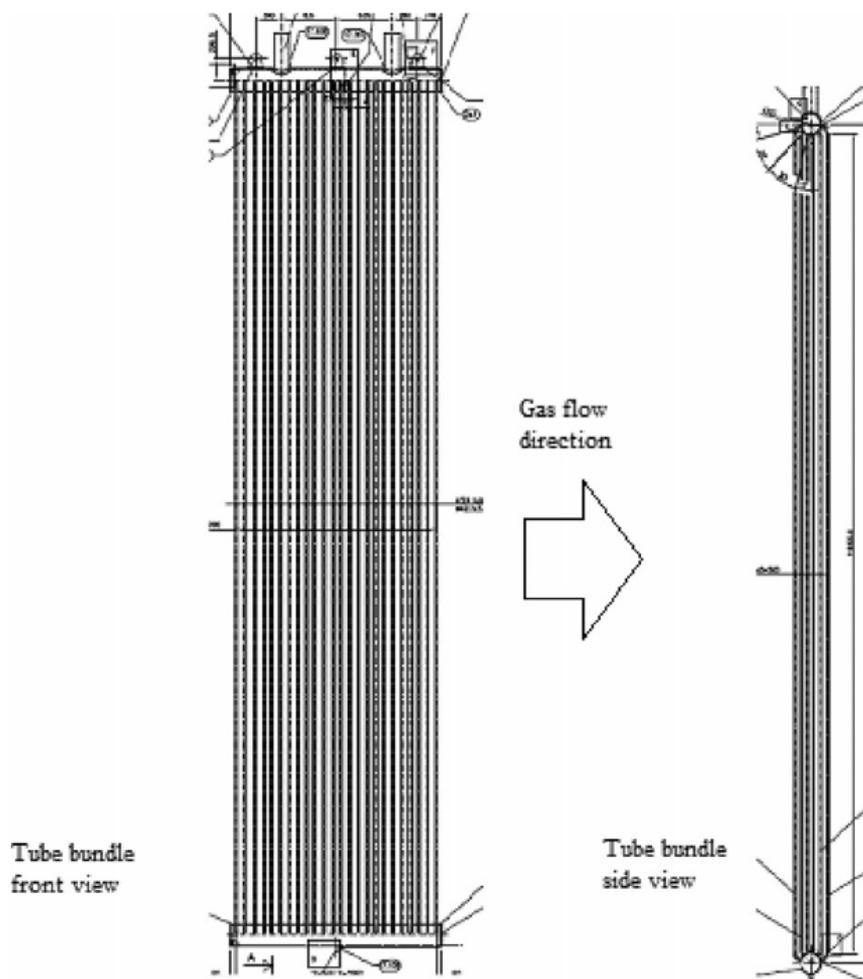
**Figure 17. Heat exchanger in Ait Baha, Morocco [62].**
