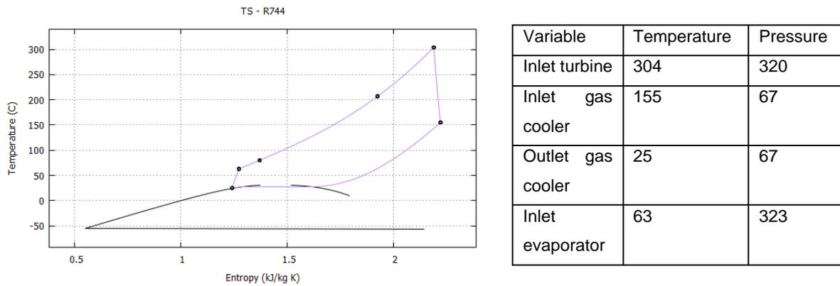
**Figure 26. T-s diagram and process data of tCO<sub>2</sub> Rankine cycle.**
