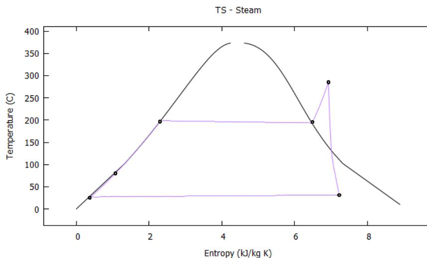
**Figure 21. T-s diagram of the Rankine cycle.**
